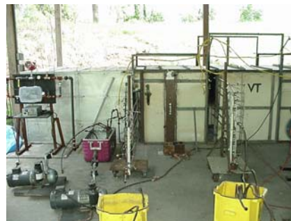
Compartment and hallway rig at BFRL
