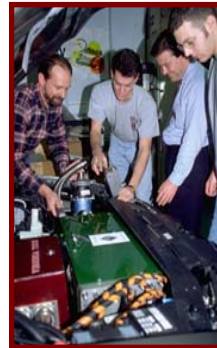
Students and professors work on a fuel cell stack in the Center for Automotive Fuel Cell Systems.
