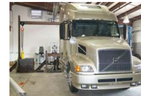
Test Rig for Evaluating the Kinematics and Dynamics of Heavy Truck Suspensions
