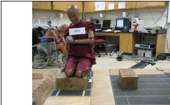
Figure 2: Positioning of the ATD and the impact block prior to fall initiation.
