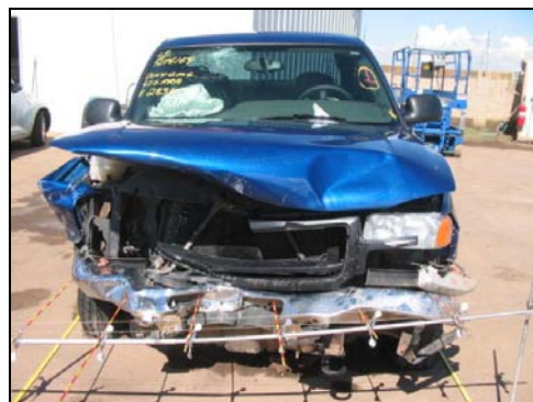
Figure 12. Case 2005-76-009 Small overlap frontal crash with another vehicle
