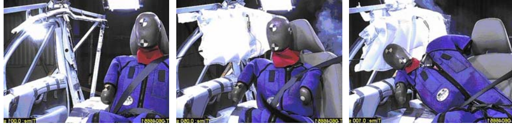
Figure 10. Photographs (flipped) at 1, 50 and 100 ms from tests conducted for this study with a belted WorldSID interacting with an inflatable curtain at 90 degrees and \Delta v 50 km/h.
