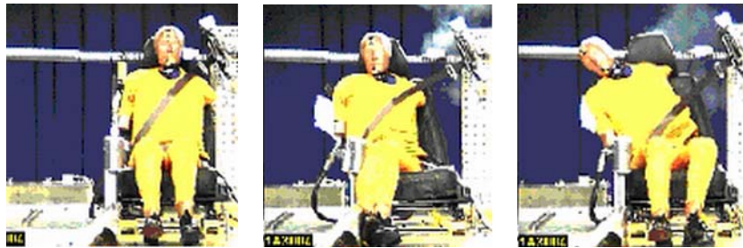
Figure 8. Photographs taken at 1, 75 and 150 ms from the Bostrom et al 2005 side support airbag test with a BioSID spring spine at 90 degrees and \Delta v 24 km/h.
