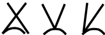
Figure 1. Three versions of altered 3-point belt geometry, criss cross, V4 and rucksack.
