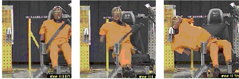
Figure 7. Photographs taken at 1, 75 and 150 ms from the Bostrom et al 2005 reference test with a BioSID spring spine at 90 degrees and \Delta v 24 km/h. The HIC indicated a severe head injury.
